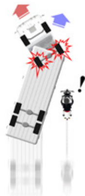
拖車頭後輪鎖死 (拖車頭車尾偏擺)
